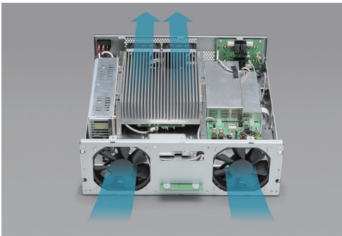
Figure 05-14. Cooling air flow
