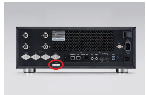
Figure 05-17. [TUNER] connector for the AH-730
