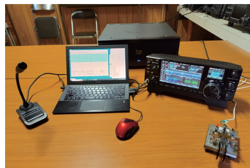
The Controller, PC, microphone, and CW paddle in front of the RF deck
