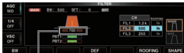
CW PITCH display (Example: 700 Hz)
