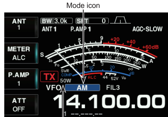
TX power readout
